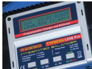
Right: Top line left side shows the digits changing from CHG to BAL with 29-minutes time lapsed and currently at 0.55 A charge rate with full 12.651 V now applied
