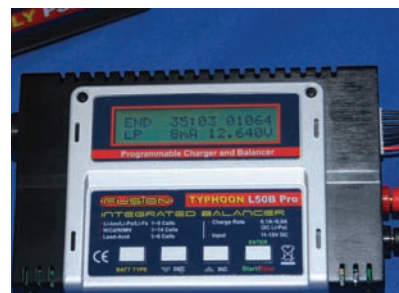
END of charge and display indicates 35.03 minutes duration and now trickle charging at 8 mA
