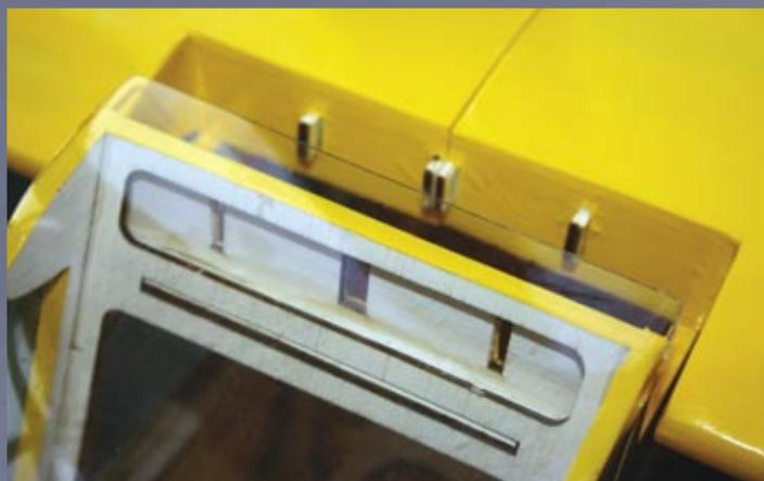
Wing LE fitting has three mounting lugs to hold wings in place
