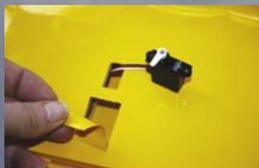
Gaining access to refit the lose aileron servo mounting plate
