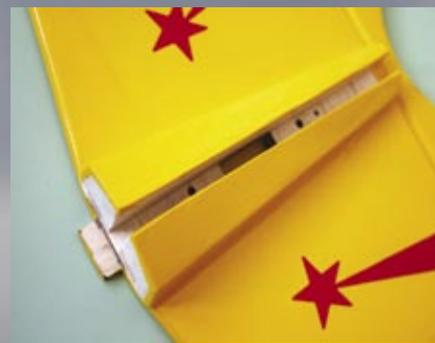
The stabiliser has an unusual screw fitting enabling removal for tight packing and transportation
