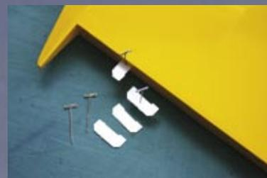
Inserting the aileron fibre hinges
