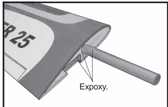
□ 2) Remove the brace when satisfied with its fit in each wing half. Coat both sides of one half of the dihedral brace with 30 minute epoxy. Next, pour some epoxy into the dihedral box in one wing panel. Make sure you cover the top and bottom as well as the sides of the dihedral brace. Use enough epoxy to fill any gaps.
