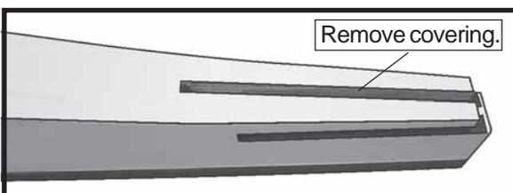
□ 3) Slide the stabilizer into place in the pre-cut slot in the rear of the fuselage. The stabilizer should be pushed firmly against the front of the slot.
