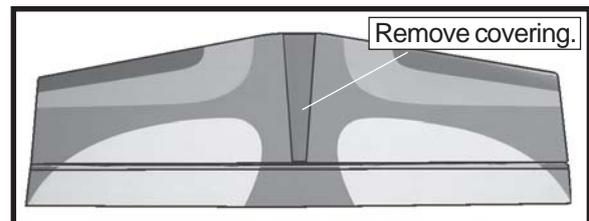
**!** *When cutting through the covering to remove it, cut with only enough pressure to only cut through the covering itself. Cutting into the balsa structure may weaken it.*
