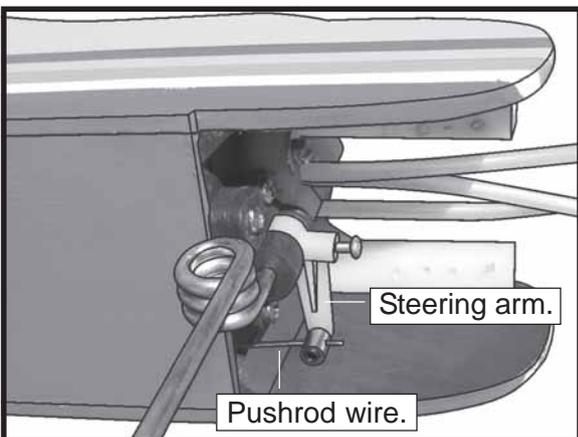
**INSTALLING THE NOSE GEAR WHEEL.**
