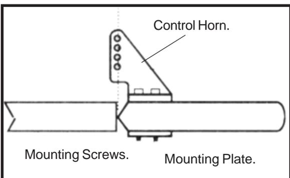
□ 3) Using a 1.5mm drill bit and the control horns as a guide, drill the mounting holes through the rudder halves.
