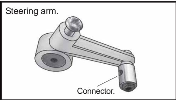
Adjust the nose gear steering arm until the arm is parallel with the fire wall.
