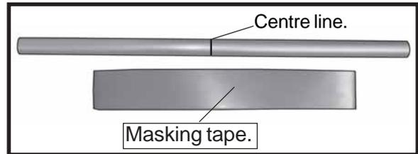
□ 1) Test fit the wing tube into each wing half. The brace should slide in easily up to the centreline that you drew. If not, use 220 grit sandpaper with a sanding block and sand down the edges and ends of the brace until it fits properly.
