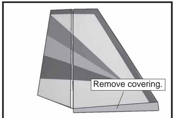
□ 3) Remove the stabilizer. Using a modeling knife, remove the covering from below the lines you drew. Also remove the covering from the bottom edge of the stabilizer and the bottom and top edges of the filler block. Leave the covering in place on the sides of the filler block.
