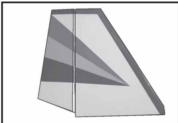
□ 1) Slide the vertical stabilizer into the slot in the top of the fuselage. The bottom edge of the stabilizer should also be firmly pushed against the top of the horizontal stabilizer.
