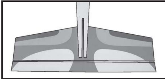
□ 8) After the epoxy has fully cured, remove the masking tape or T-pins used to hold the stabilizer in place. Carefully inspect the glue joints. Use more epoxy to fill in any gaps that may exist that were not filled previously and clean up the excess using a paper towel and rubbing alcohol.
