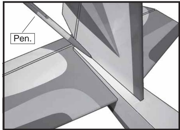
□ 2) While holding the vertical stabilizer firmly in place, use a pen and draw a line on each side of the vertical stabilizer where it meets the top of the fuselage.
