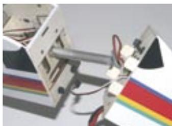
The nose locates on an ali tube, four lugs and is retained by four nylon bolts.
