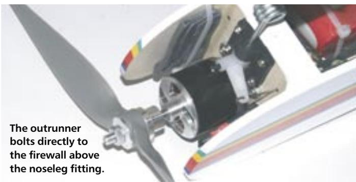
The outrunner bolts directly to the firewall above the noseleg fitting.
