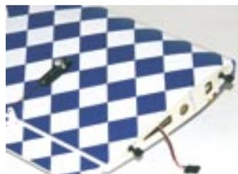
The wing joiner is an ali tube and identical nylon bolts hold the panels in place.
