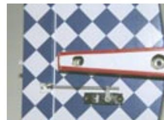
Tail servos are mounted in the flying surfaces - two bolts hold the tail on.
