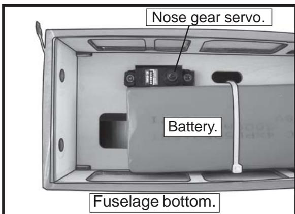
**INSTALLING THE STEERING ARM SERVO.**
