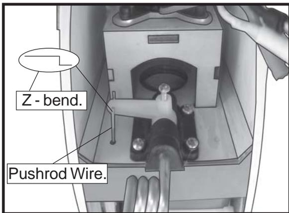
**INSTALLING THE BATTERY- NOSE GEAR SERVO .**
