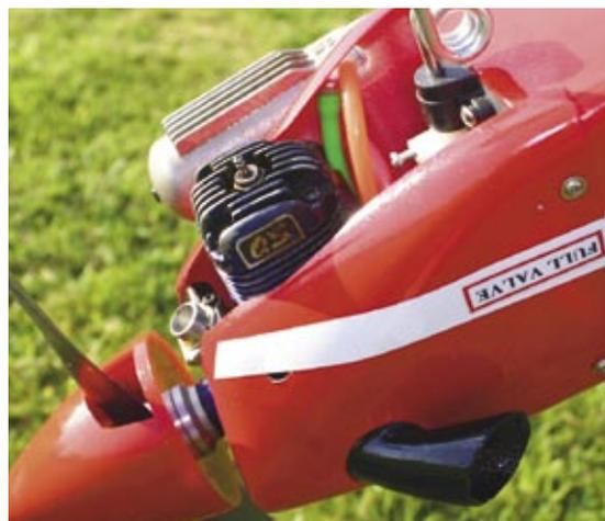
*The inverted engine installation is, perhaps, the only drawback with the model, though it does at least maintain the clean lines of the cowl.*
