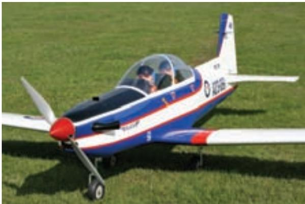
*The spinner supplied isn't well balanced so I fitted one of the Irvine metal backplate examples.*
