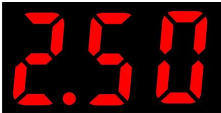
5. Servo / ESC manual test mode, short press or long press the increase key to increase the output signal pulse width value, the maximum output pulse width signal is 2.50ms.
