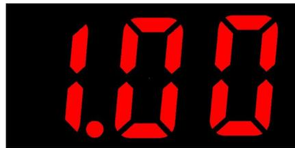
6. Servo / ESC manual test mode, short press time mode function key to enter the servos / ESC automatic test mode, the minimum output pulse width signal at this time: 1.00ms.
