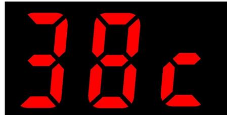
11. Correct access LM35 temperature sensor, the screen will display the current real-time temperature, such as the current temperature of 38 degrees Celsius, the digital display screen is displayed as "38c".
