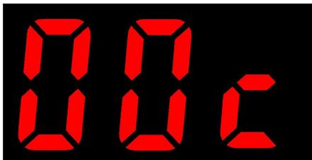
10. The receiver signal out of control to monitor the alarm mode, short press time mode function key, you can enter the temperature measurement and over-temperature alarm mode; If you do not access or not properly connected to the LM35 temperature sensor, the screen will show "00c", "c" for the unit of degrees Celsius.
