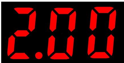
7. In the servos / ESC automatic test mode, the digital display screen digital display from 1.00 to 2.00 loop Happy Valley, then the output pulse width signal: 2.00ms.
