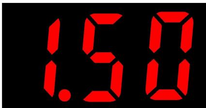
3. Servo / ESC manual test mode, the digital display shows "1.50" then the output pulse width signal is 1.50ms (unit: ms).
