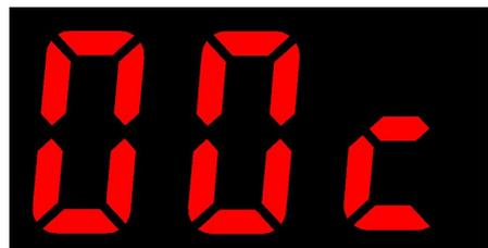
13. Temperature measurement and over-temperature alarm mode, short press or long press the lower key to decrease the temperature alarm threshold, the minimum to 0 ° C, display said "00c".
