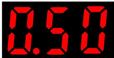
4. Servo / ESC manual test mode, short press or long press to reduce the key, can reduce the value of the output signal pulse width, the minimum output pulse width signal is 0.50ms.
