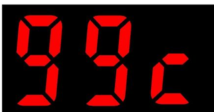
14. Temperature measurement and over-temperature alarm mode, short press or long press the increase key to increase the temperature alarm value, the maximum is 99 ° C, display said "99c".
